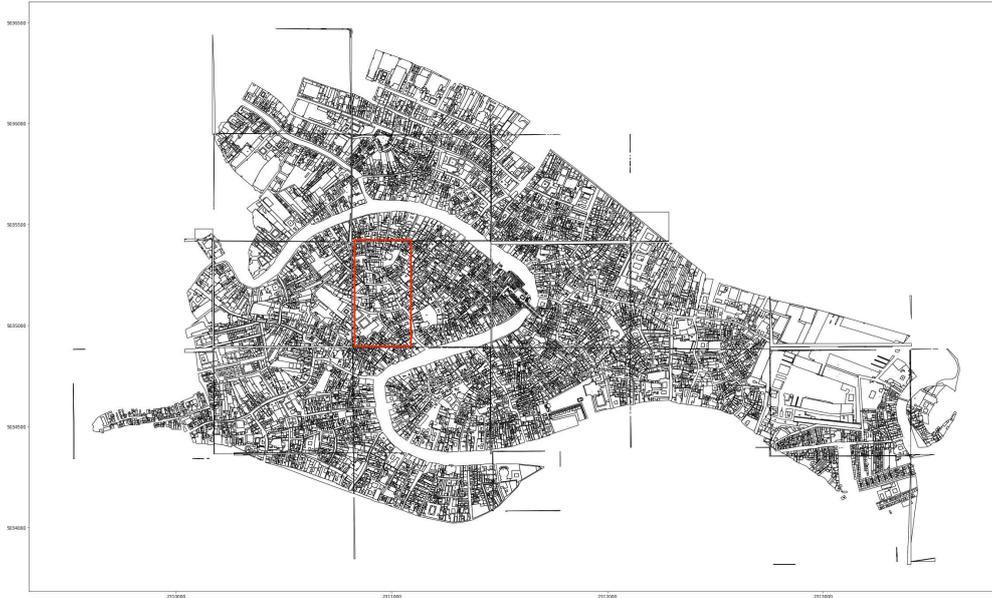
Figure 13: Visualization of the results of the automatic extraction of parcels. The red rectangle indicates the parcels used as training data for the segmentation network.
