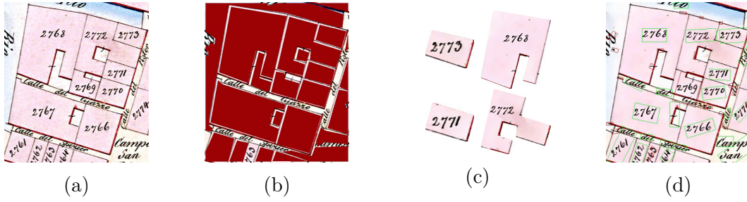
Figure 2: Sample of results : (a) original image, (b) polygon approximation of parcels, (c) extracted parcels and (d) identifiers localization
